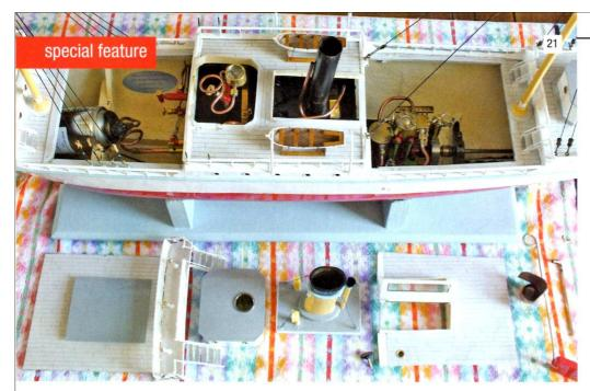
and propshaft in action. Photo 21 is of the model separated from it superstructure components and this also shows the final internal arrangements very nicely.
