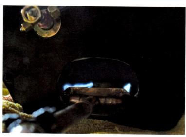
Photo 12. The final diameter of the poker holes was determined by testing with the boiler. These were eventually optimised at 1.9mm diameter which gives sufficient 'comph' to maintain pressure at about 30 to 35psi with the engine running at a speed to realistically propel the yacht, but without wasting steam and gas by 'blowing off'. However, it must be said that the final hole size was determined after practical on the water steaming trials subsequent to this last picture.
